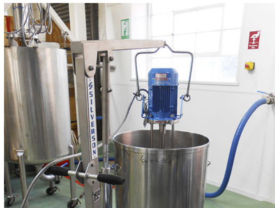
Industrial mixer used for producing graphene flakes by shear exfoliation. © Trinity College Dublin. Portrait: © Samuel Sanchez, El País.
