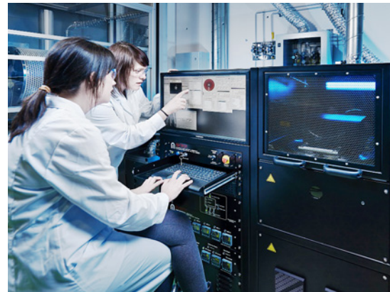
Production of 6-inch graphene on an AIXTRON BM Pro system. These are transferred onto flexible polyethylene naphthalate substrates by Graphenea, and then integrated into a flexible organic light-emitting diode (13 × 13 cm) by Philips. © Aixtron Ltd.
