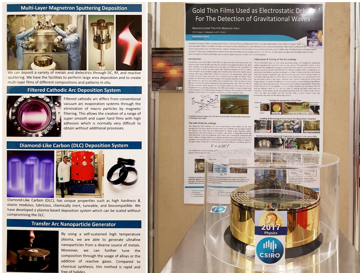
Figure 9: Visit to the labs of CSIRO Lindfield. Besides the Graphene labs, the participants also saw the advanced material deposition capabilities offered by the thin film lab (left). In particular, high precision gold electrostatic drivers were fabricated at this facility for the Laser Interferometry Gravitational Observatory (LIGO); gravitational waves were observed with these detectors, recognised by the 2017 Nobel Prize being awarded for this work.
