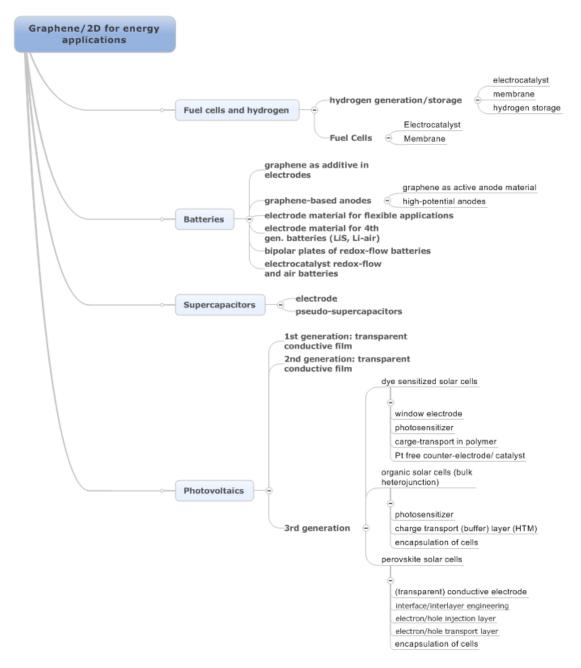
Figure 48: Energy related application areas of graphene/2D materials.
