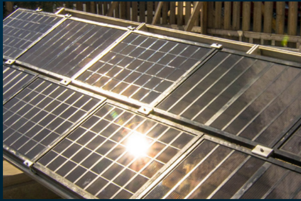
The world's first outdoor demonstration of a solar farm with 4.5 m 2 graphene-perovskite panels. Credit: Nature Energy
