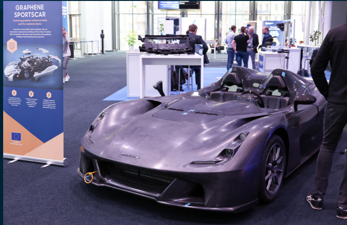
The Dallara Stradale sports car uses graphene composites in the body for fire retardancy and better shock absorption during collisions. Credit: Graphene Flagship
