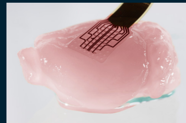
Neural interface device to record neuron activity. Credit: ICN2
